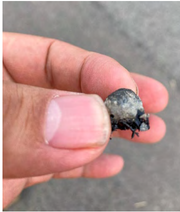
Figure 4-2. Photo. Chip Pulled Out from the Core Surface.
