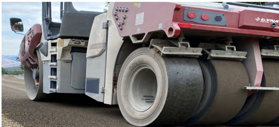
Figure 3-8. Photo. Combination Roller (Combo): Steel Drum (front) and Pneumatic Wheels (back).
