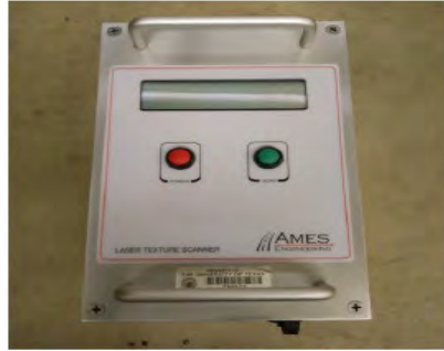
Figure 2-5. Photo. AMES Laser Texture Scanner Model 9300 (Source: Zuniga Garcia, 2017)
