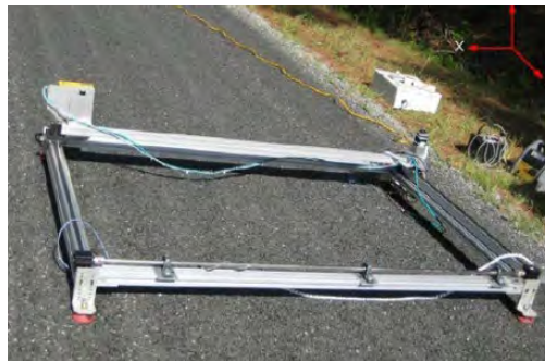
Figure 2-8. Photo. 3-D Laser Profiler (Source: Kim et al., 2012).
