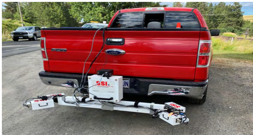
Figure 3-13. Photo. SSI Profiler Mounted on a Pickup Truck.
