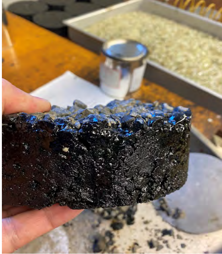
Figure 4-19. Photo. Asphalt Dripping after Tilting of a Sample in the Oven Overnight.
