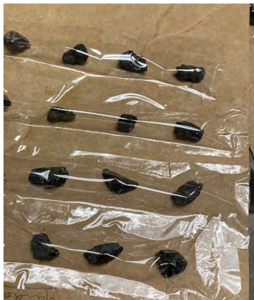
Figure 4-3. Photo. Extracted Chips from SR 127 in the Field.
