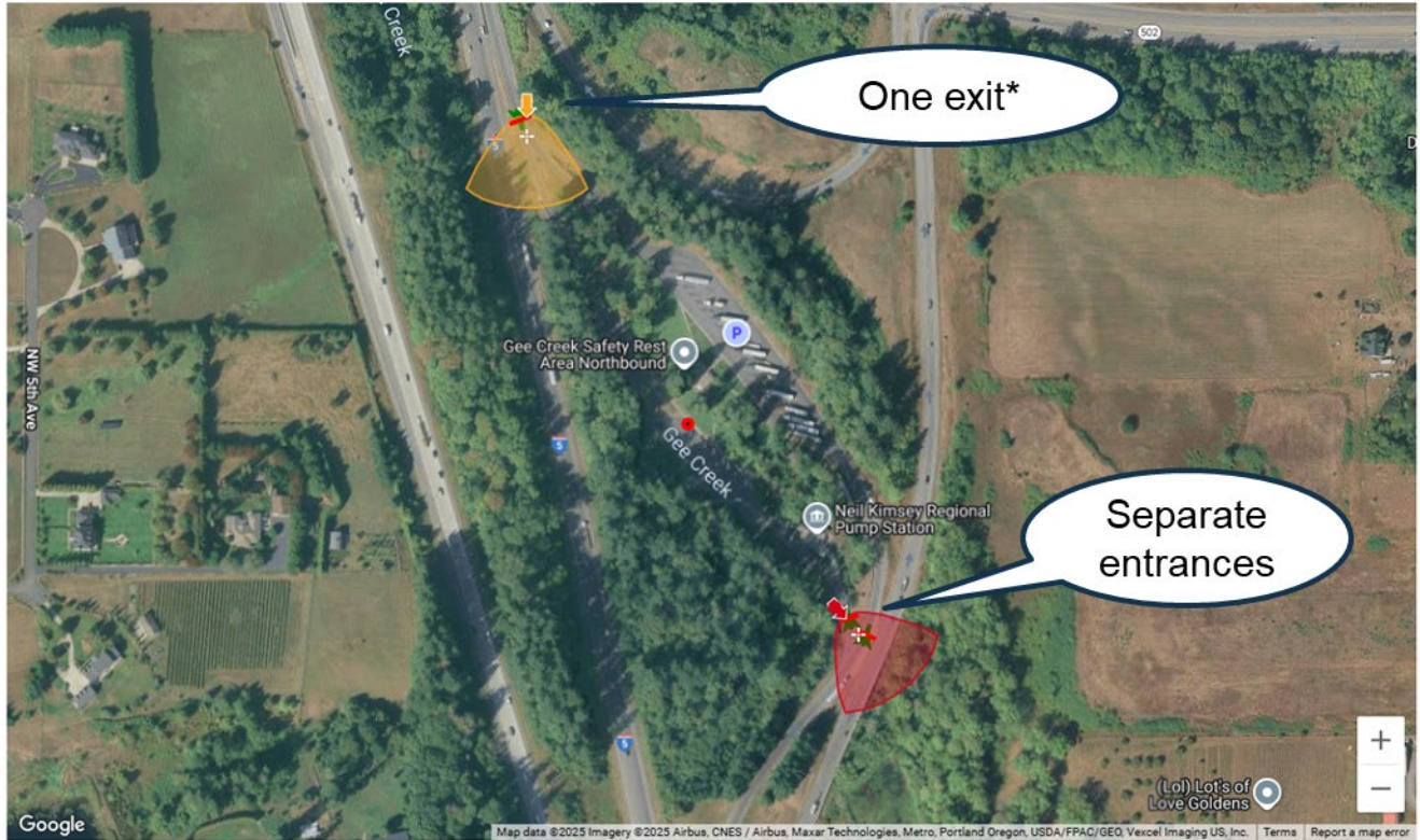
Figure 5-9 Example of vehicle classification challenges at Gee Creek NB site with separate entrances but a shared exit, where overlapping truck, RV, and general-purpose vehicle movements reduce in/out detection accuracy.
