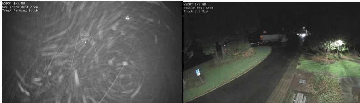
Figure 5-11 Severe environmental conditions at Gee Creek NB (left) and camera view obstruction caused by vegetation at Toutle River (right).
