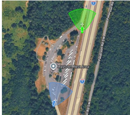
Figure 4-1 Installation layout of in/out counting sensors at the entrance and exit of the Maytown site.
