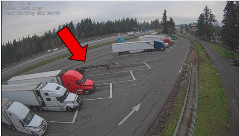
Figure 5-8 Example of a trailer occupying multiple parking spaces, which can lead to discrepancies between sensor-based counts and actual parking availability.
