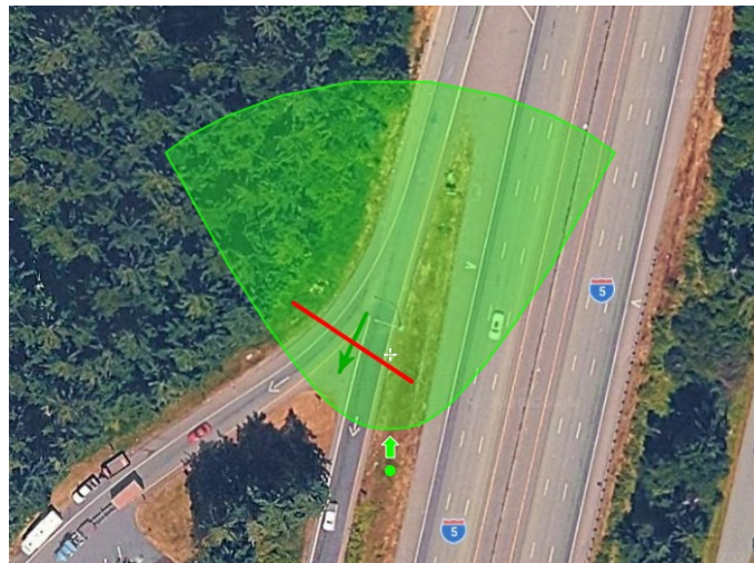
Figure 4-2 Example of the screenline configuration at the entrance of the Maytown site. The red line indicates the virtual screenline used by the sensor to detect vehicles crossing the entrance, while the shaded area represents the sensor's detection coverage.
