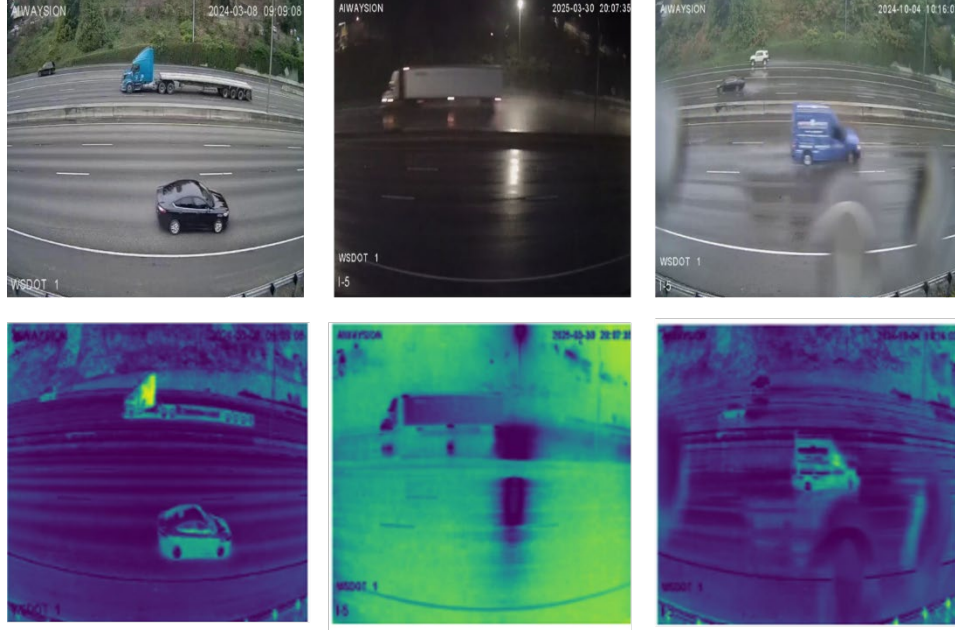
Figure 34. Visual comparison of input images (top) and extracted feature maps (bottom).
