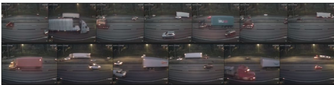
Figure 30. Example of day-to-night translation using CycleGAN. The nighttime images are generated by translating daytime images using the CycleGAN model.
