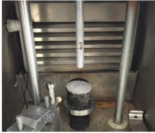
Figure 5 Ice layer rupture test (Ma et al. 2016)
