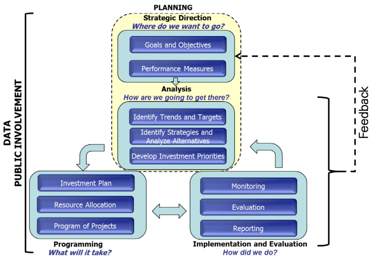
Figure 4. Flowchart. Framework for performance-based planning and programming. (Source: Federal Highway Administration, Performance-Based Planning and Programming Guidebook, September 2013.)
