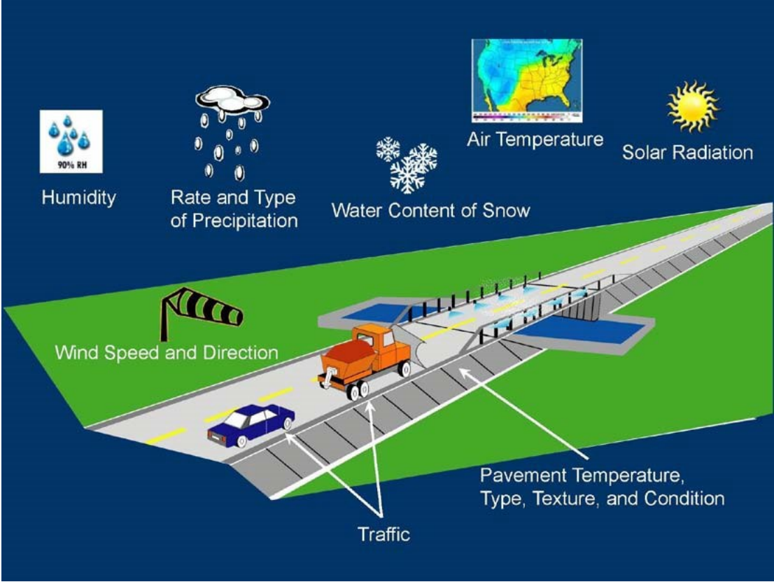
Figure 1-1 Schematic diagram illustrating the major parameters that influence deicer performance and pavement friction (Muthumani et al. 2015).
