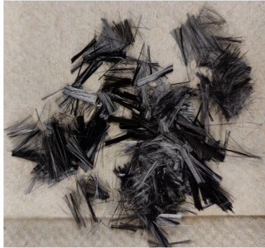
Figure 4-2: Chopped up carbon fiber (10-mm length) for the experiment
