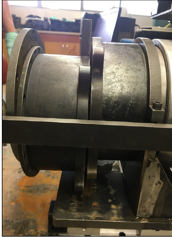
FIGURE 44. Direct shear test set-up.
