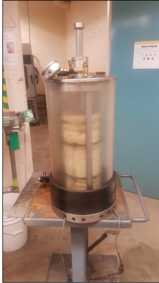
FIGURE 49. Triaxial test set-up.
