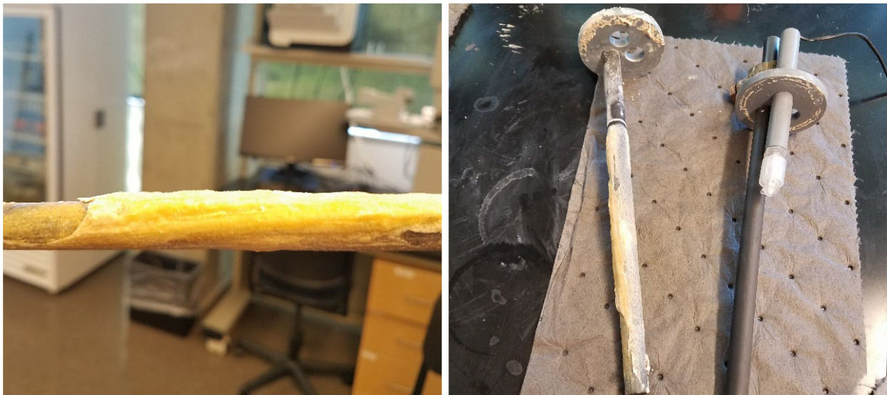
Figure 45. Photo. Post-treatment electrodes. Left photo: Cathode. Right photo: Left = cathode, Right = anode (experiment 4).
