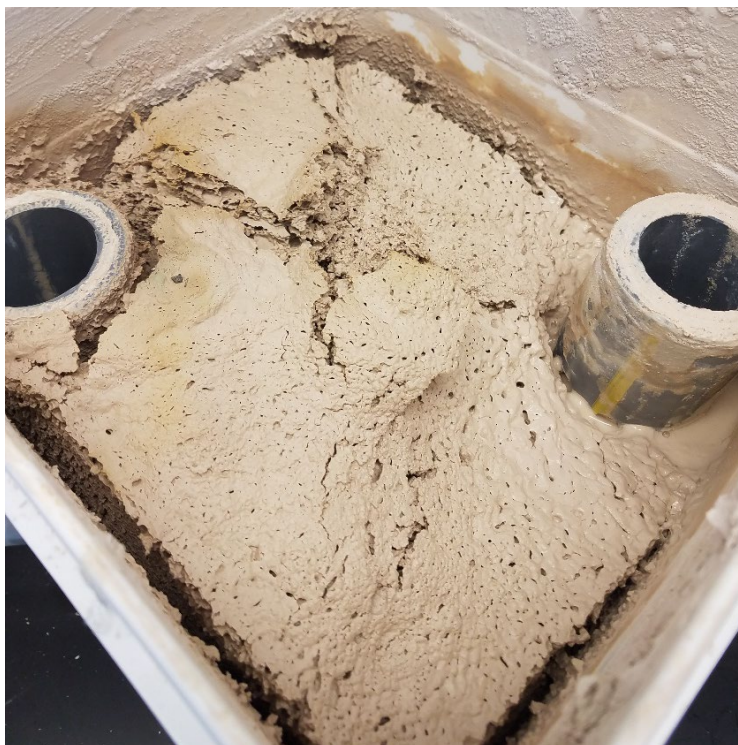
Figure 38. Photo. Post-treatment soil surface with swelling induced changes in soil structure (experiment 1).
