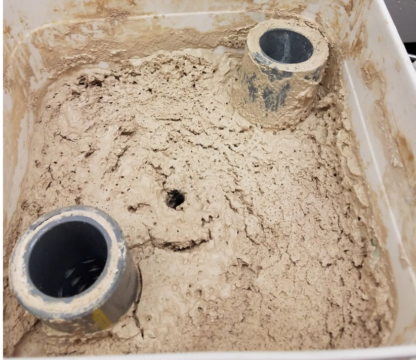
Figure 44. Photo. Post-treatment soil surface riddled with sponge-like voids (experiment 4).
