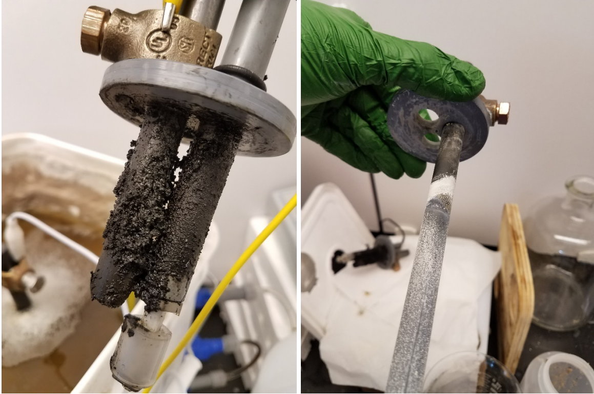
Figure 43. Photo. Post-treatment electrodes. Left = anode. Right = Cathode (experiment 3).
