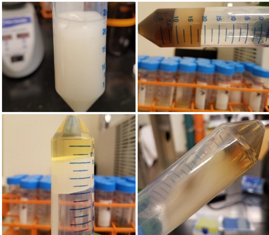
Figure 41. Photos. Surfactant induced saponification during post-treatment sample centrifugation (experiment 3).
