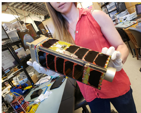
Figure 3. The 3U Cubesat built at UW for delivery to NASA, Sept 2019.
